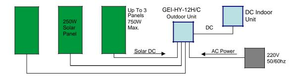
Like all DC-Inverter air conditioners, the ACDC12 compressor runs on DC power converted from AC power. But this special solar air conditioner can also accept DC power directly from solar panels, without needing an inverter, controller, or batteries. The solar DC power directly replaces an equivalent amount of AC power from the power company and can cut daytime energy costs for air conditioning or heating by 80% or more.
